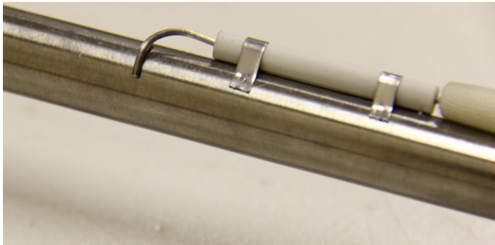
Figure 2.19 A typical spot welded thermocouple on the heater element external surface.
