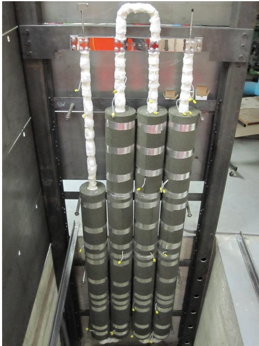
Figure 2.7 Heater element with Foamglass ® solid thermal insulation.
