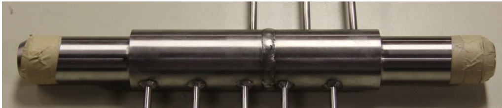
Figure 2.15 Photo of the test section showing the welded region.
