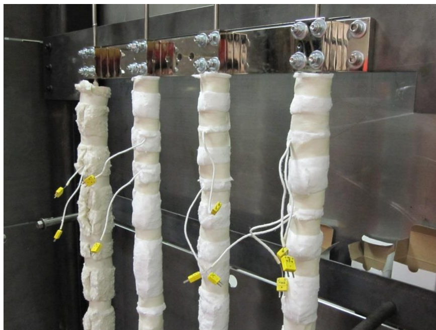
Figure 2.6 Heater element with Superwool ® insulation.
