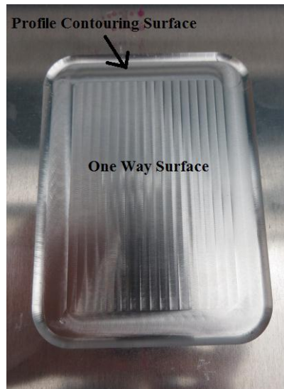
Figure 7.21 Two different surfaces inside the pocket
