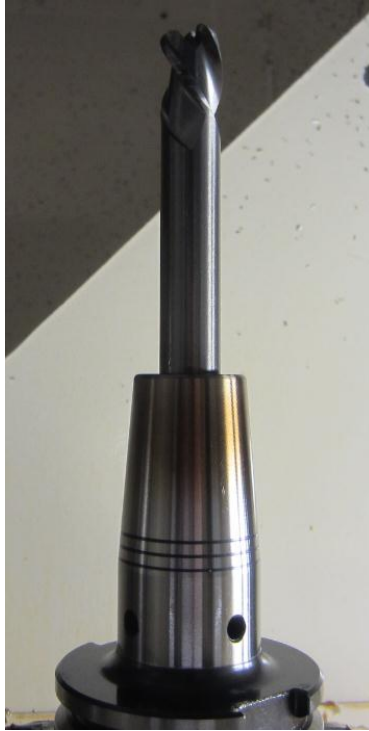
Figure 6.7 Overview of the shrink-fit holder and cutting tool
