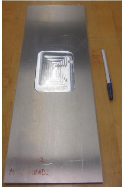
Figure 7.6 The pocket milled sheet
