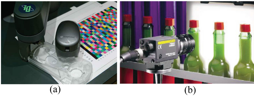
Figure 6.4 Machine vision system for (a) color recognition [213] and (b) detection of “under-filled” bottles in a beverage production line [214].
