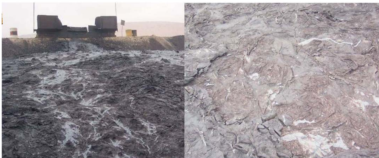
Figure 11.11. Presence of matte in the RHF slag dam site.
