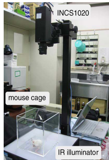
Figure 2.7 The set-up used by Nie et al. [2010] (© 2010, IEEE)
