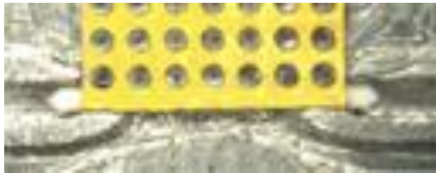
Figure 2-13: Top view of a fabricated iSINRD guide (continuous metal wall, circular profile).
