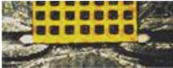
Figure 2-14: Top view of a fabricated iSINRD guide (continuous metal wall, square profile).
