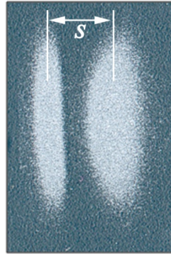
Figure 3.5: Optical image of typical velocity calibration wear scars with the offset s indicated.
