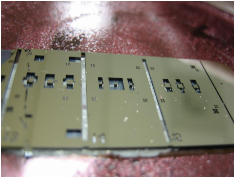
Figure 4-18: Photograph of several VOA accelerometer devices after the 500 \mu\text{m} backside DRIE of SOI for the case of VEM approach.
