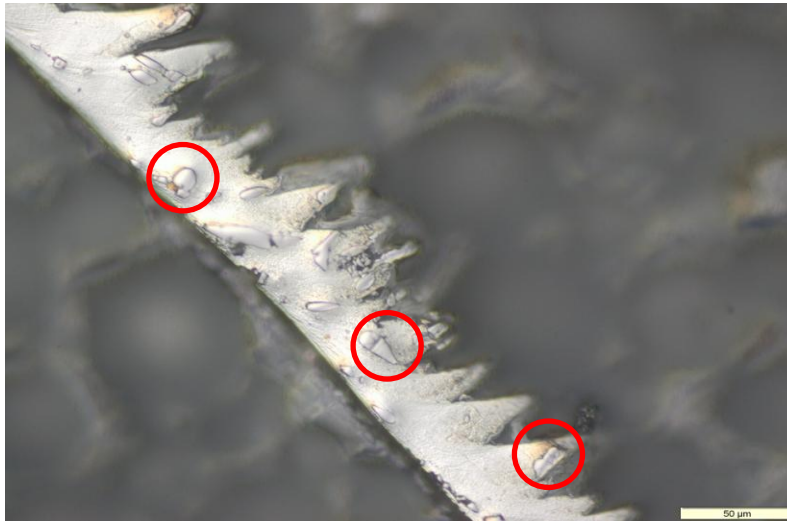
Figure 2.16- Chip morphology when the surface temperature is at 1000°C
