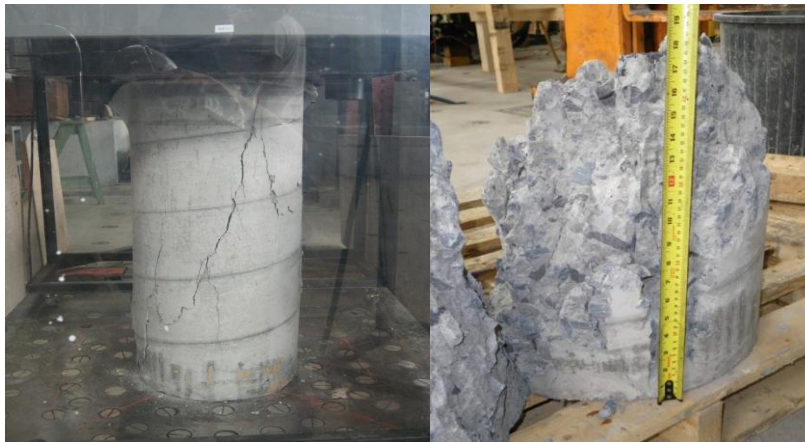
Figure 3-2: Mass concrete cylindrical specimen (400mm x 800mm)
