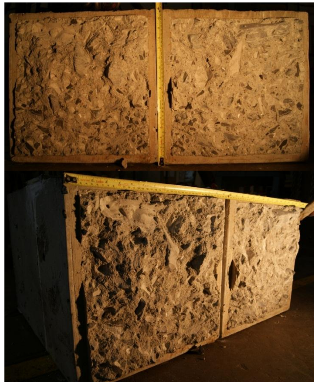
Figure 3-6: Modulus of Rupture Failure Plane (Specimen E)
