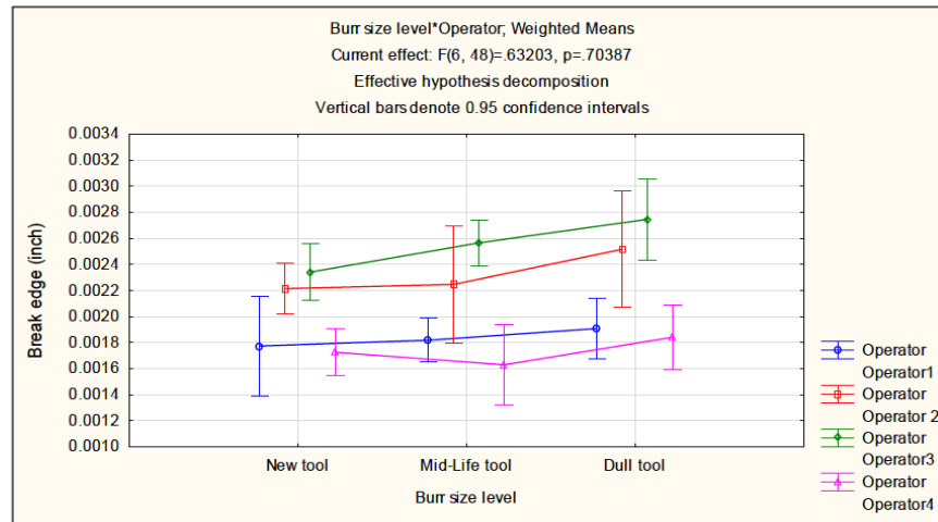
Figure 6-15: Effect of burr size and operator on break edge (Part B)
