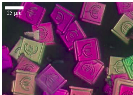
Figure 3.5 Example of a micro-structured square shaped magenta to green optically variable pigment displaying a Euro symbol. Image taken from [66].
