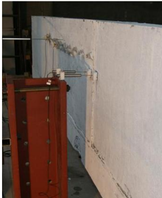
Appendix B Figure 5: Displacement at End of Loaded Barrier and Adjacent Barrier
