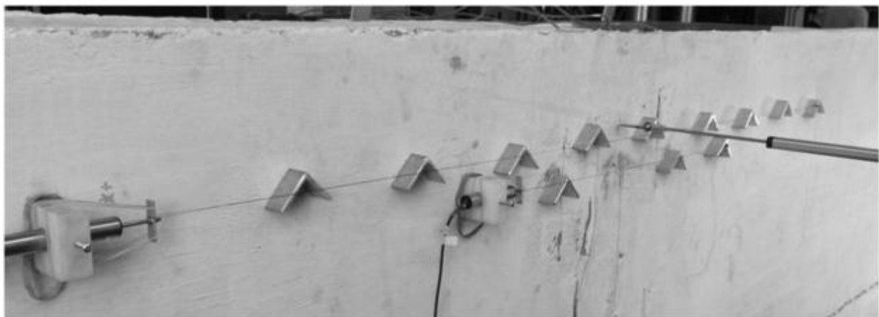
Figure 5-33: Barrier Longitudinal Deformation Sensors
