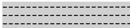
Figure 5.5 Discretization of the superconducting layer of one tape into magnetically coupled line elements in the IM model. Although it is pictured as a straight line, the domain is actually curved.
