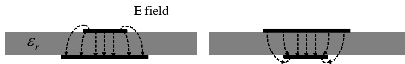
Figure 1.2: Electrical field plots on the A plane
