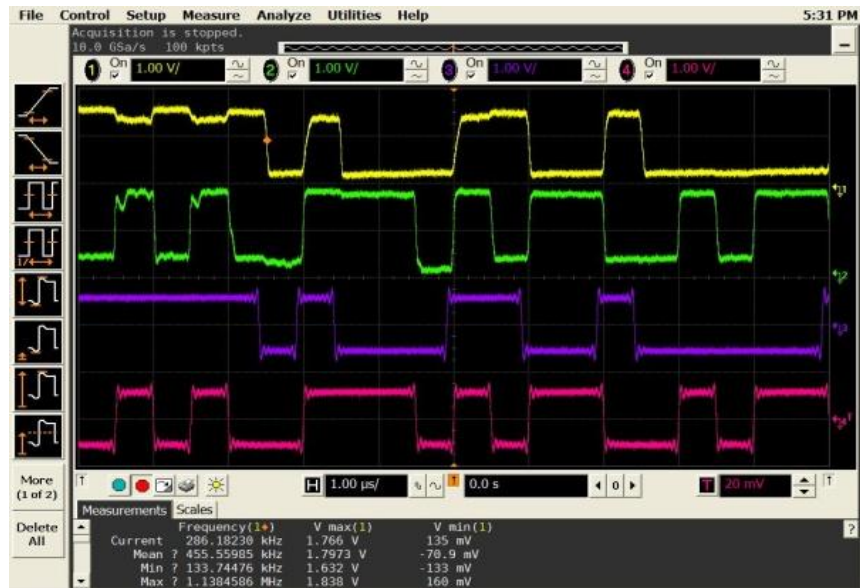
Figure 8.12: Comparison of the received (1 st and 2 nd waveforms) and transmitted I/Q signals (3 rd and 4 th waveforms)
