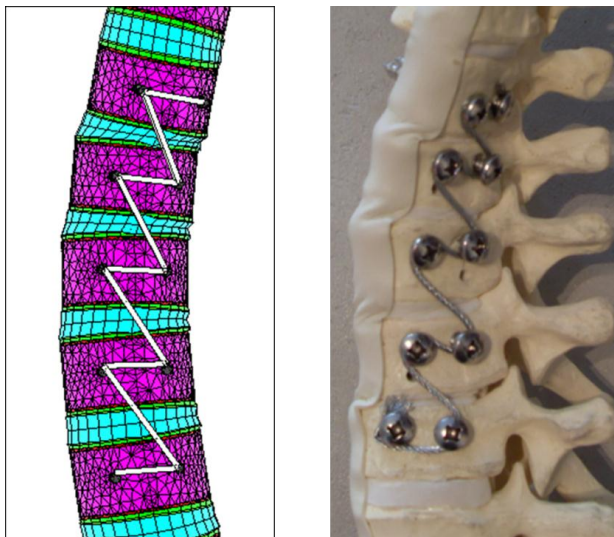
Figure 6.10: Example of agreement between in silico and in situ manipulation of spinal alignment by the 3D corrective tether
