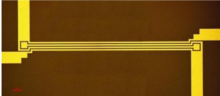
Figure 5.36 An SEM photo of the fabricated Lange coupler before bonding wires assembly.
