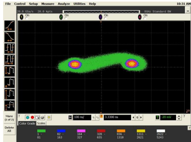
(b) Constellation of 10-Mbps BPSK signal.
