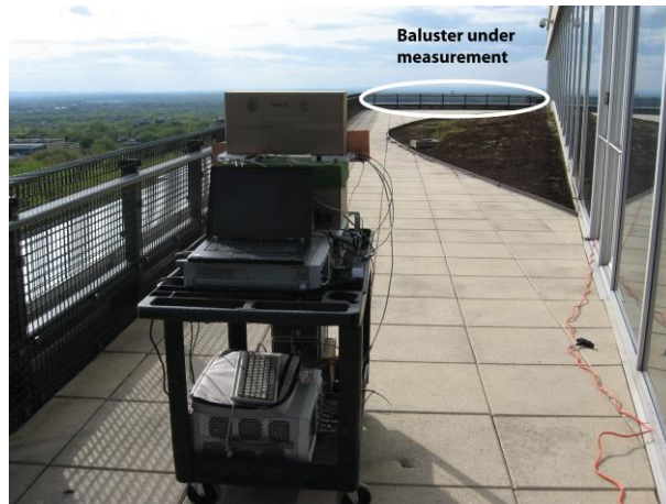
Figure 3.44 Experiment setup for measuring the distance of a baluster.
