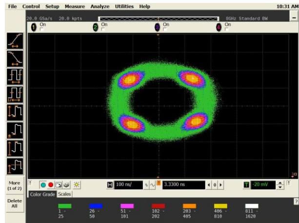
(b) Constellation of 10-Mbps QPSK signal.
