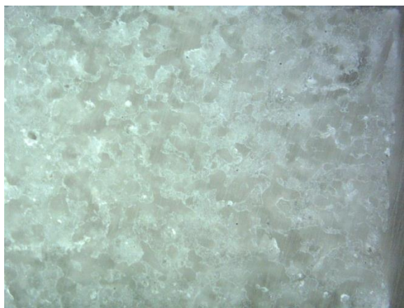
Figure 6-9 : Micrograph of cross-section porous hydroxyapatite
