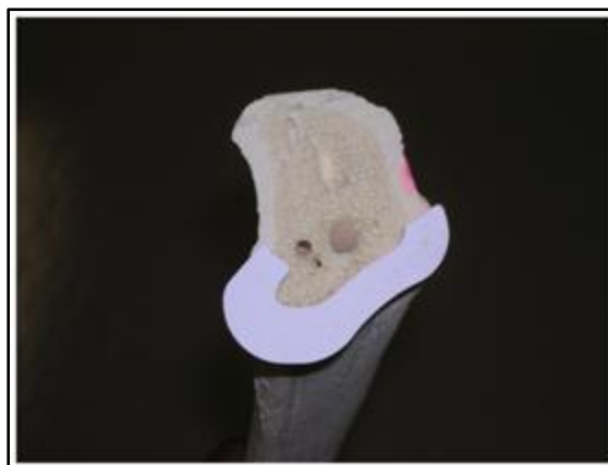
Figure 6-11: Porous personalized bioceramic implant
