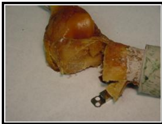
Figure 4-5 : Mode of Failure in the construct for load-to-failure loading
