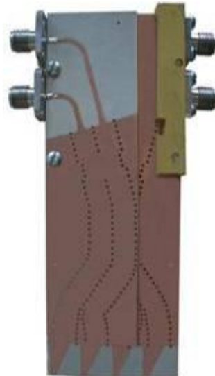
Fig.16. Photography of the developed four ALTSA element antenna array fed by a 4 x4 Butler matrix made of SIW structure.
