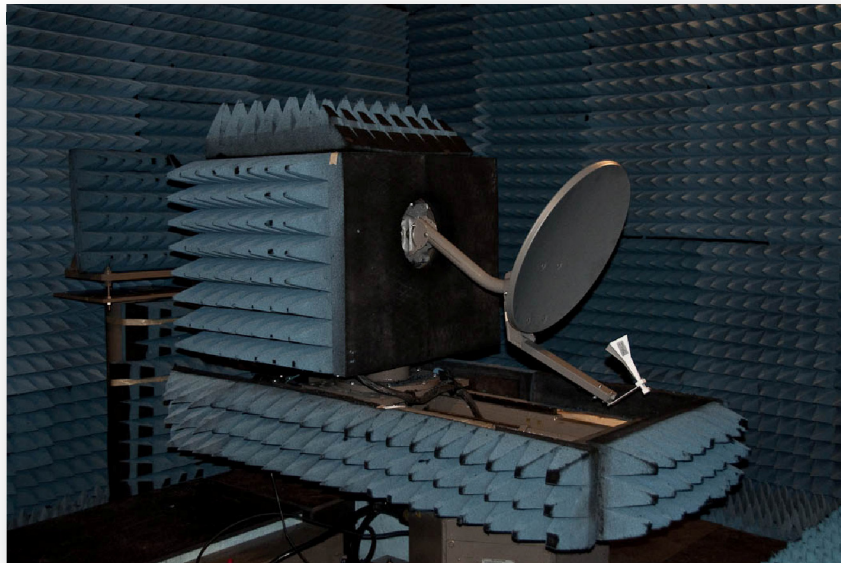
Figure 4.2 Reflector antenna measurement.
