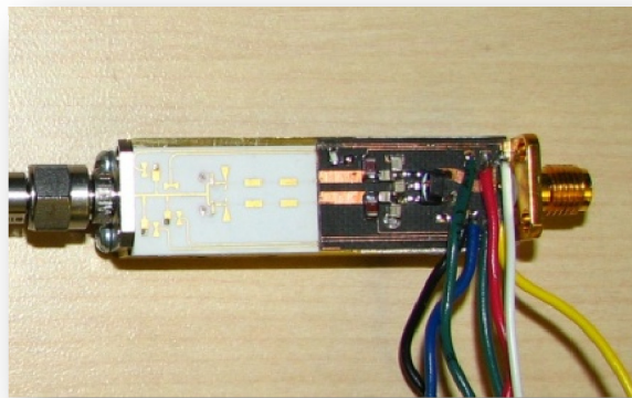
Figure 3.33 Photograph of the proposed 35 GHz self-oscillating mixer.
