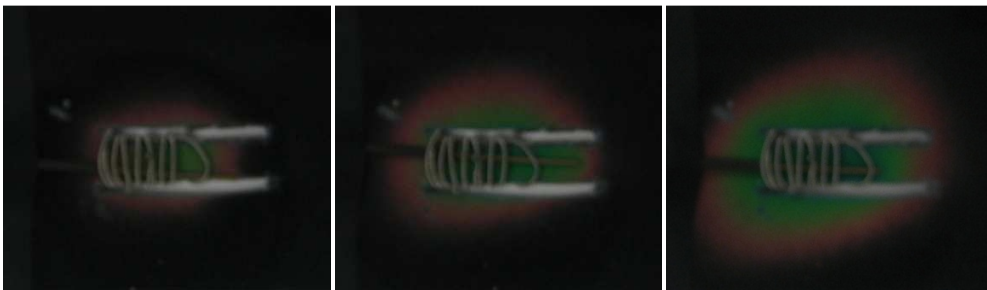
Figure 5.34 L = 10 mm, images taken after 2, 5 and 10 minutes of RF delivery
