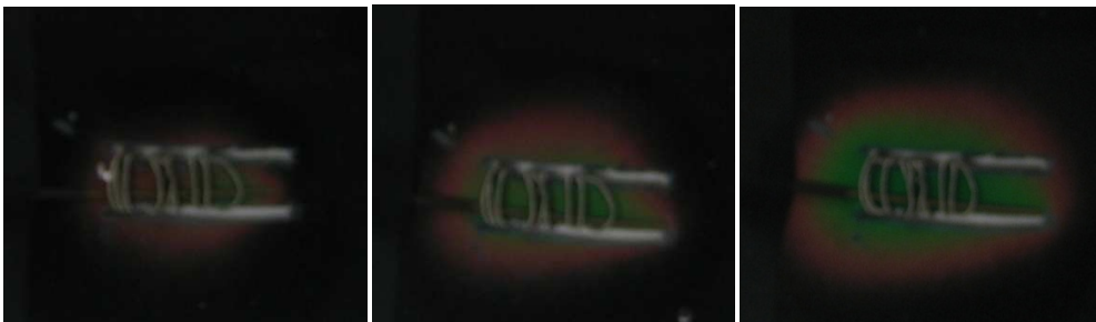
Figure 5.35 L = 15 mm, images taken after 2, 5 and 10 minutes of RF delivery
