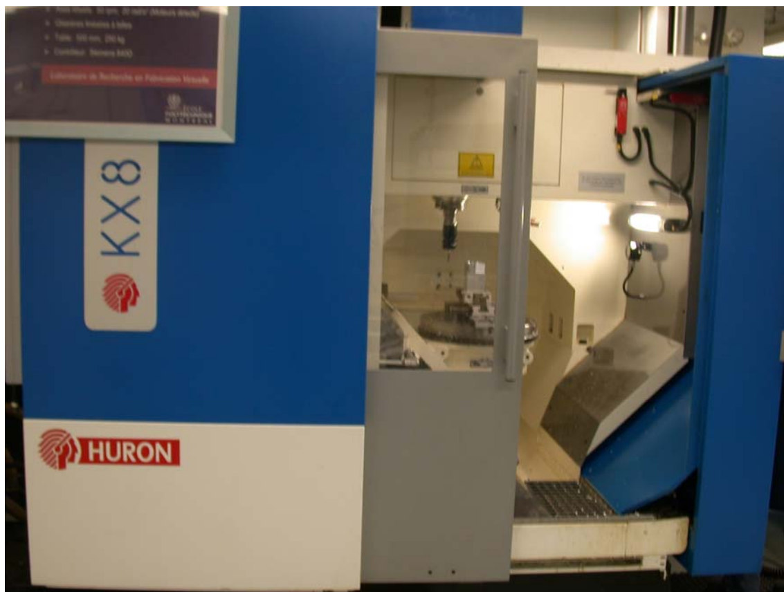
Figure 3-3: Centre d'usinage HURON KX 8 Five.
