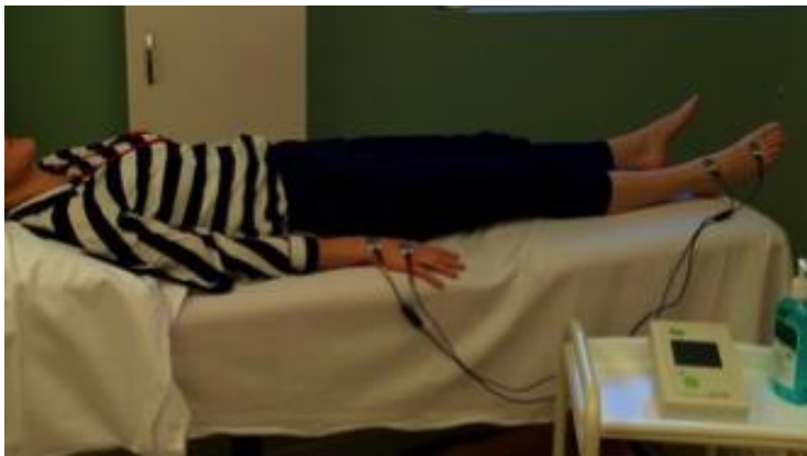
Figure 4.1: Bioimpedance spectroscopy: standard whole body electrode positions
