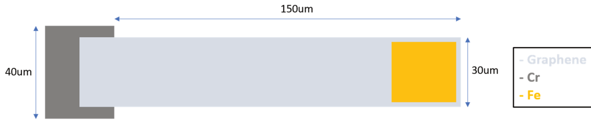
Scheme 3. Enlarged graphene micro ribbon with an iron patch.
