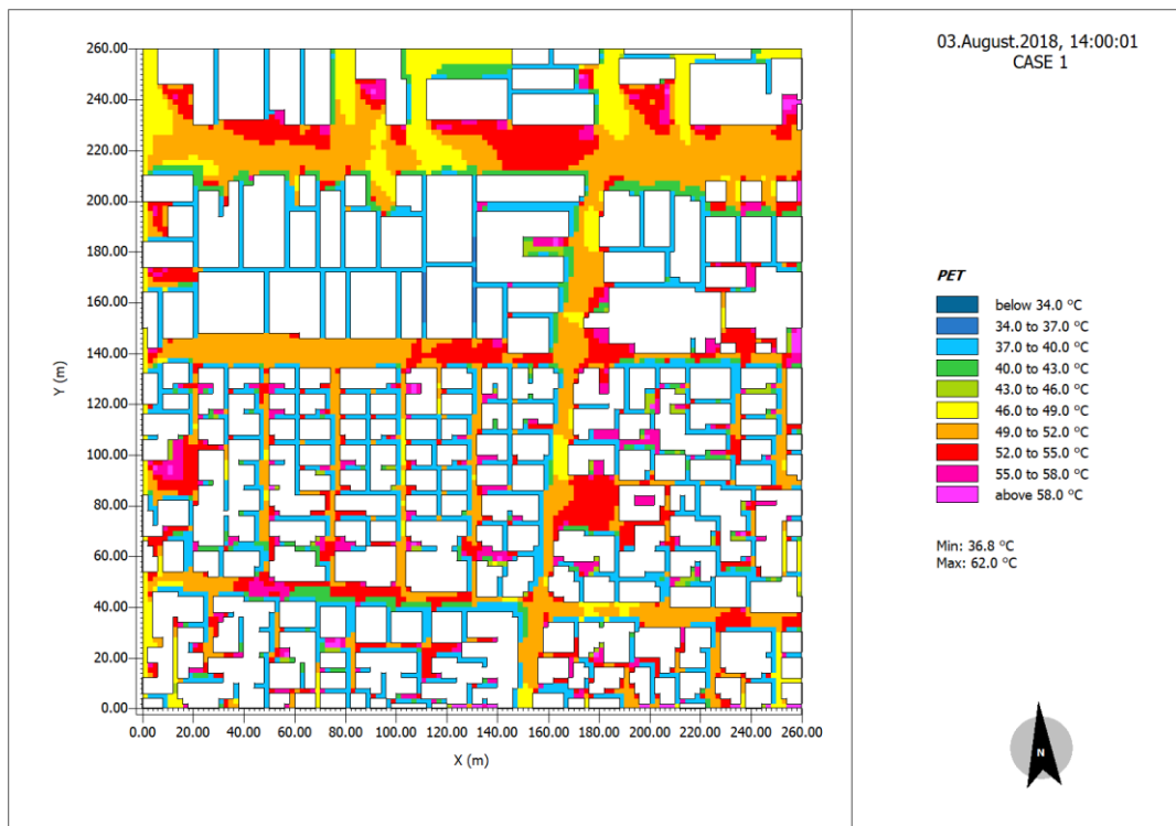
Figure 5.8 Simulated PET values at a height of 1.4 m agl for case 1 (current site configuration) at 14h on the heat wave day of 3 August 2018 (white areas: buildings).
