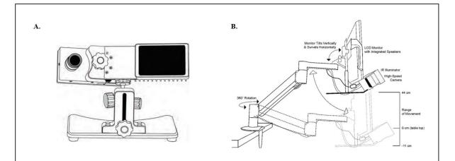
**Figure 2.5** | An image of EyeLink 1000 Plus instrument. **(A)** Front view of instrument is featured with eye camera. **(B)** Side view of instrument is composed of eye camera and monitor for stimulus presentation. The height and direction of the camera and monitor can be easily changed.
