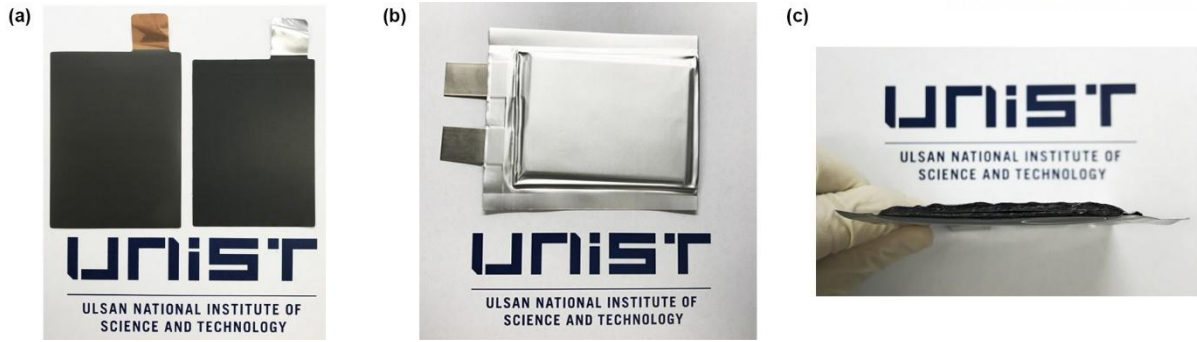
Figure 4. 3. Photographs of the pouch-type full-cell with the cell capacity of 1.2 Ah. (a) Double-sided cathode and anode for stack type pouch cell. (b) Stacking type pouch cell with the dimension of 70 mm * 90 mm * 2.5 mm. (c) Cross sectional photograph of the pouch cell.
