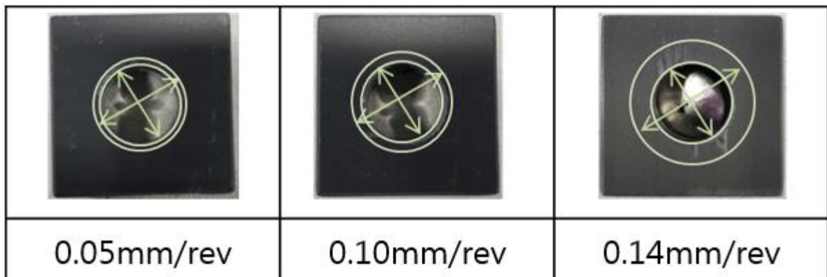
Fig. 6-8. Delamination extent according to feed in the same RPM
