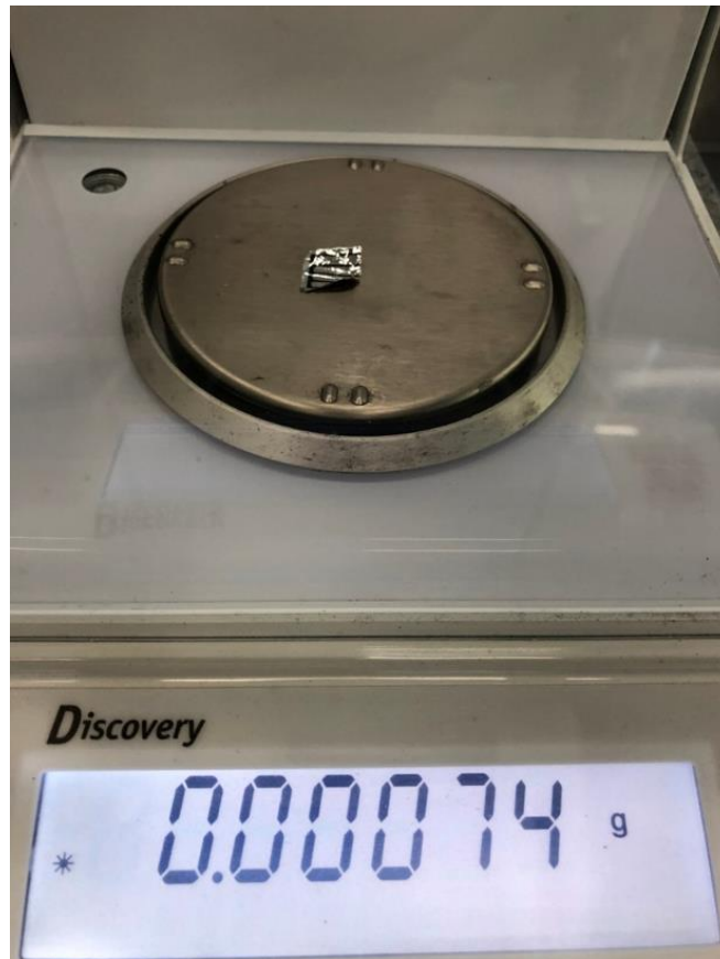
Figure 7. 12. Photograph of an ultralight PSC device on an electronic scale, demonstrating its extremely low weight. The device size is 13 mm x 13mm
