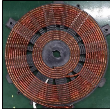
Fig. 14. IH working coil with 16 turns
