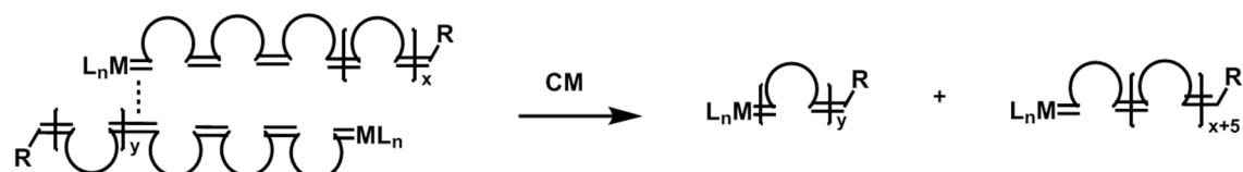
Figure 1.5. A representative mechanism for ring opening metathesis polymerization (ROMP) and examples of intramolecular chain transfer via ring closing metathesis (RCM) and intermolecular chain transfer via cross metathesis (CM).
