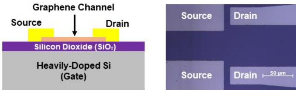
Figure 3.4 The fabricated GFET structure and its optical microscope image. The source and drain electrodes are Ti/Au (10/50 nm) and the channel width and length are both  $10 \mu\text{m}$ . [Submitted]
