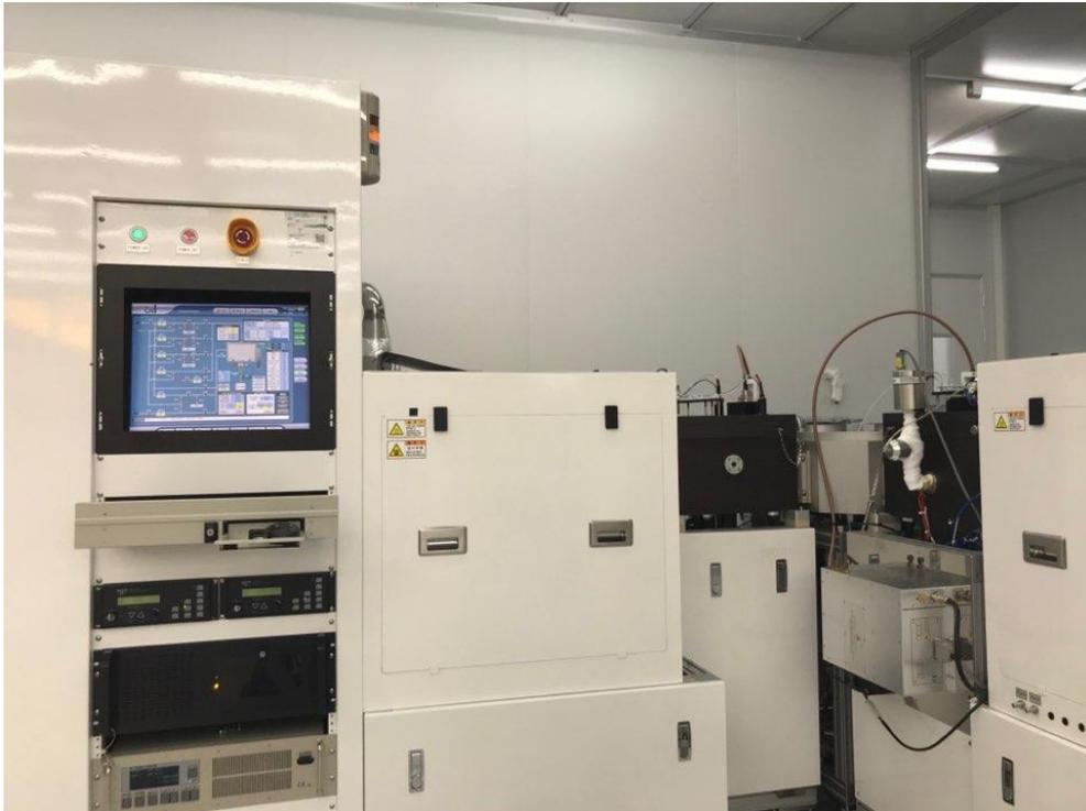
Figure 5.1 Atomic Layer Deposition (ALD) system in nanofabrication clean room in UNIST.
