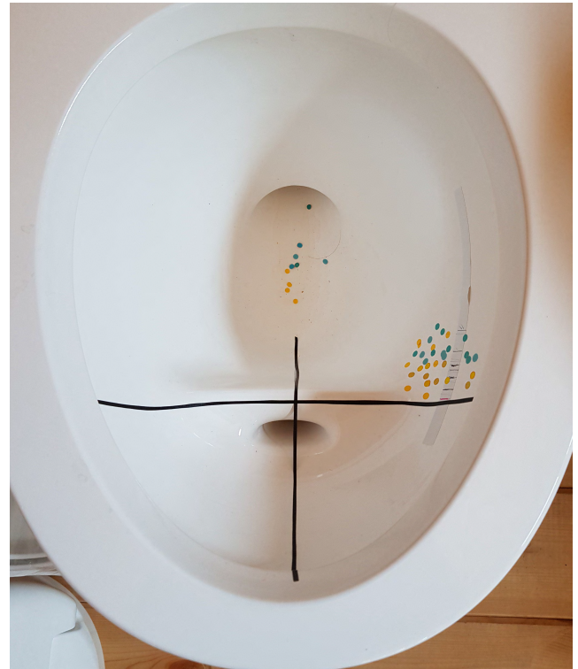
FIGURE 9. Distance preference of the urine and feces separating wall, based on the urine angle of user experiences (men = yellow, women = green).
