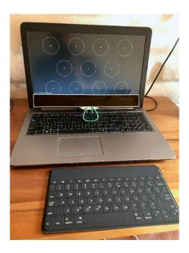
Figure 3. Computer with eye-tracking camera and remote keyboard following calibration.
