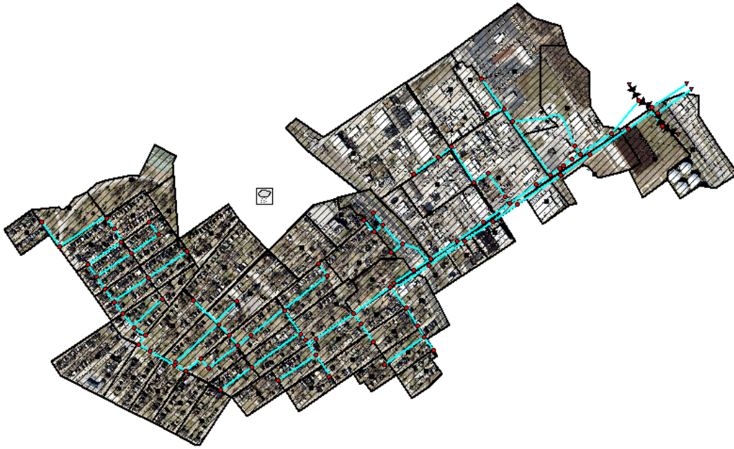
Figure 3.6. Catchment and Sewer Network With Backdrop Image
