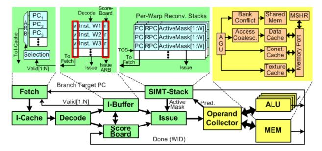
Figure 3.3: Detailed Microarchitecture Model of SIMT Core [4]
