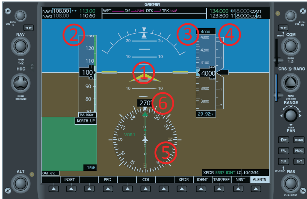
Figure 2: Parts of a PFD. Garmin shown. Others Similar. (FAA, 2012). Altered by Author.
