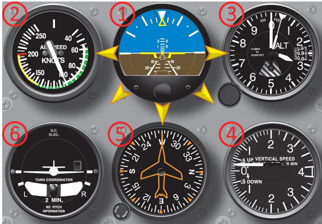
Figure 1: Standard Six Pack Instruments and Locations (FAA, 2012). Altered by Author.
