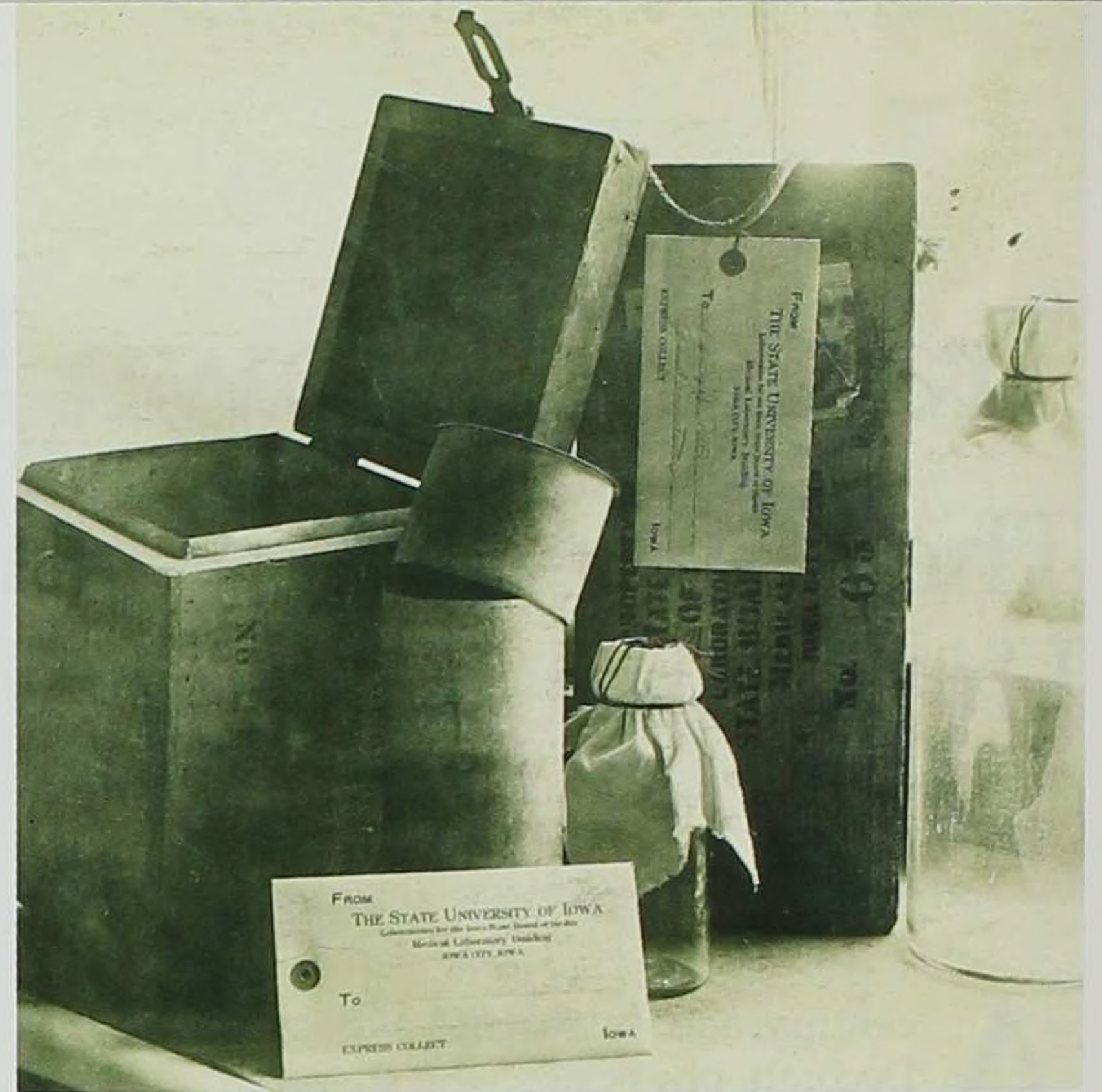
The Hygienic Laboratory repeatedly directed Iowans who wanted their well water tested to use the water collection kits provided by the lab (right), rather than salt-glazed jugs and bottles stoppered with corncobs, corks, or rolled paper (above)—all likely to contaminate the sample.
