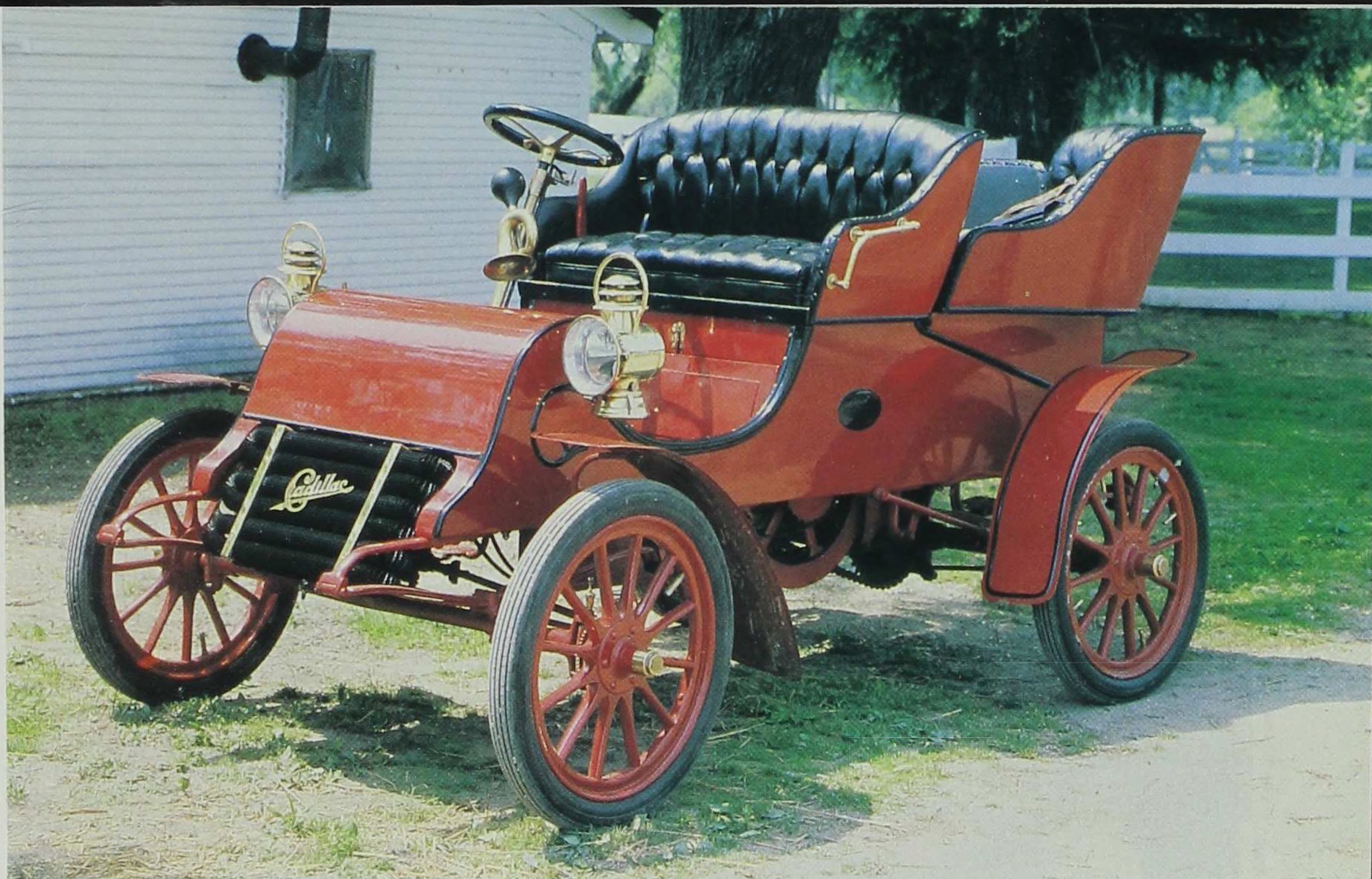
“Old Calamity” probably looked like this in 1903. Note the low-slung radiator and its exposed coils, the sloping hood, and the rear tonneau. This 1903 Cadillac runabout is owned by Donald C. Burnham of Pittsburgh, Pennsylvania.
