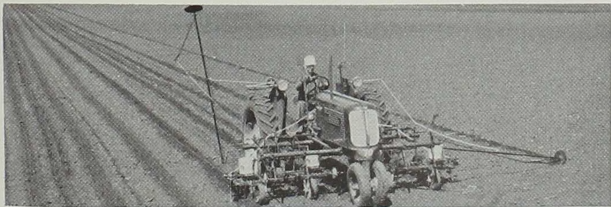
Four-row tractor planter with check rower.
