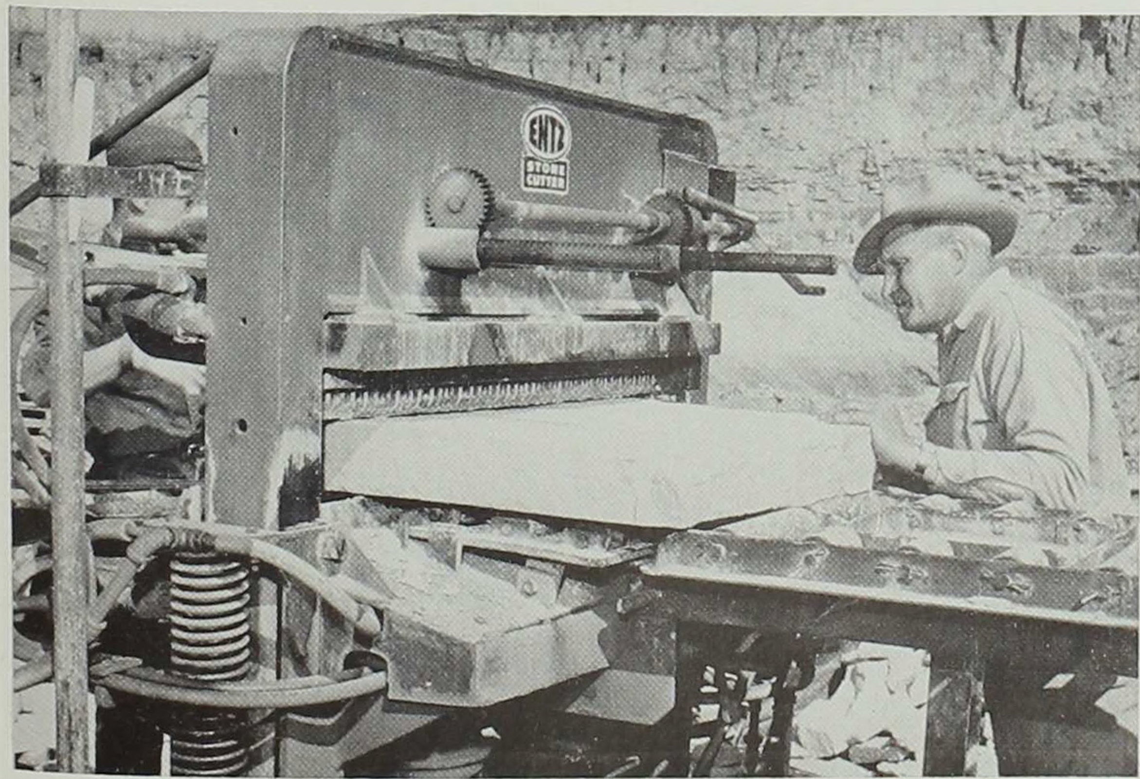
The conveyor carries the stone to this machine where it is cut into the desired size.
