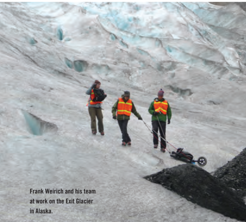
Frank Weirich (left) and student Phil Kerr check on the ground-penetrating radar unit in its reinforced transport sled.
