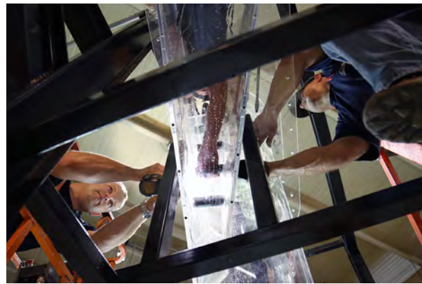
TOP: IIHR built a 1:24 scale physical model of a portion of the Ohio River near the Cardinal Power Plant.
