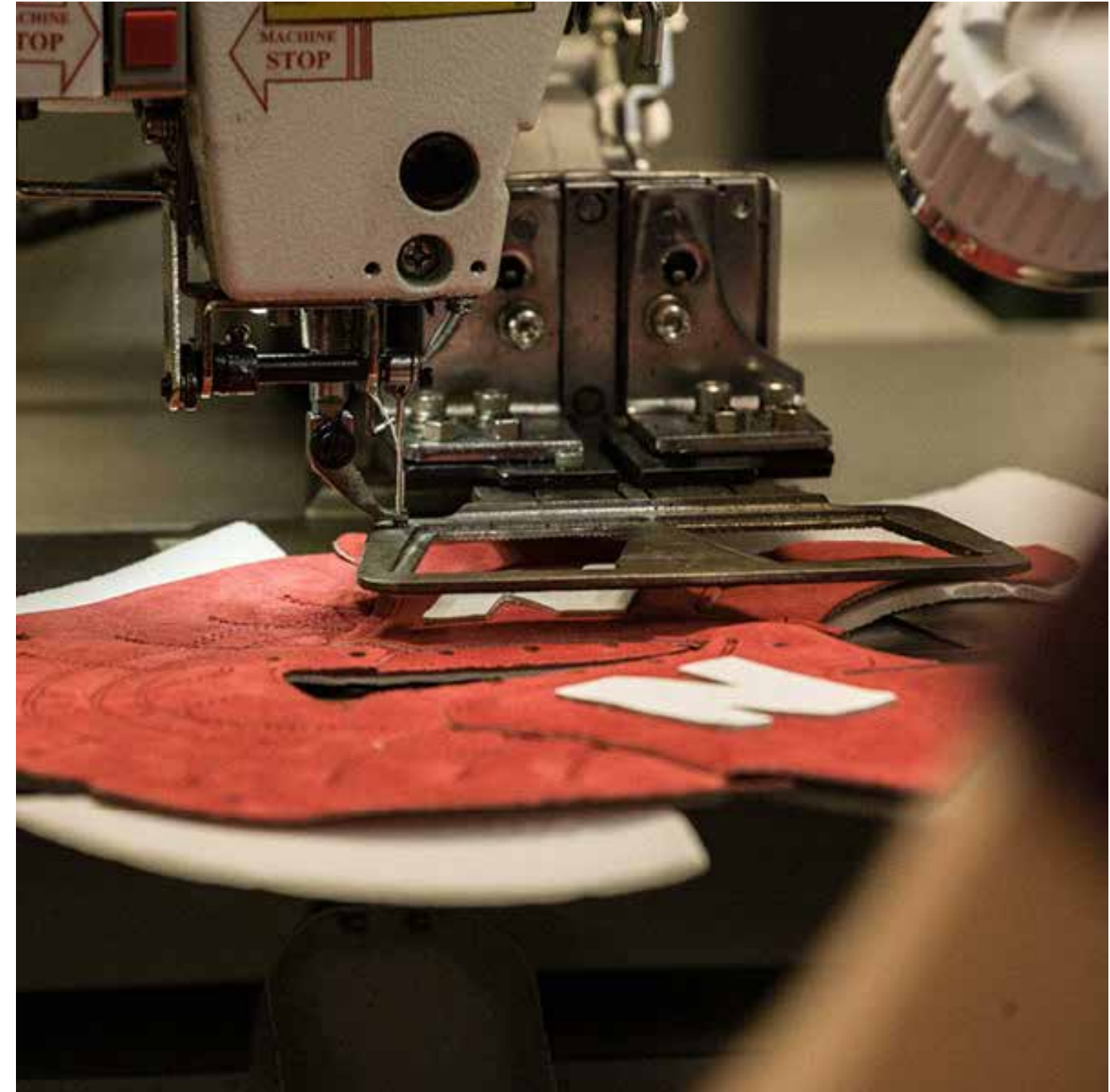
An upper being automatically stitched in a U.S. New Balance facility. This suede upper is a combination of classic footwear materials with a simplified construction, requiring less hands, pieces, and different materials.
