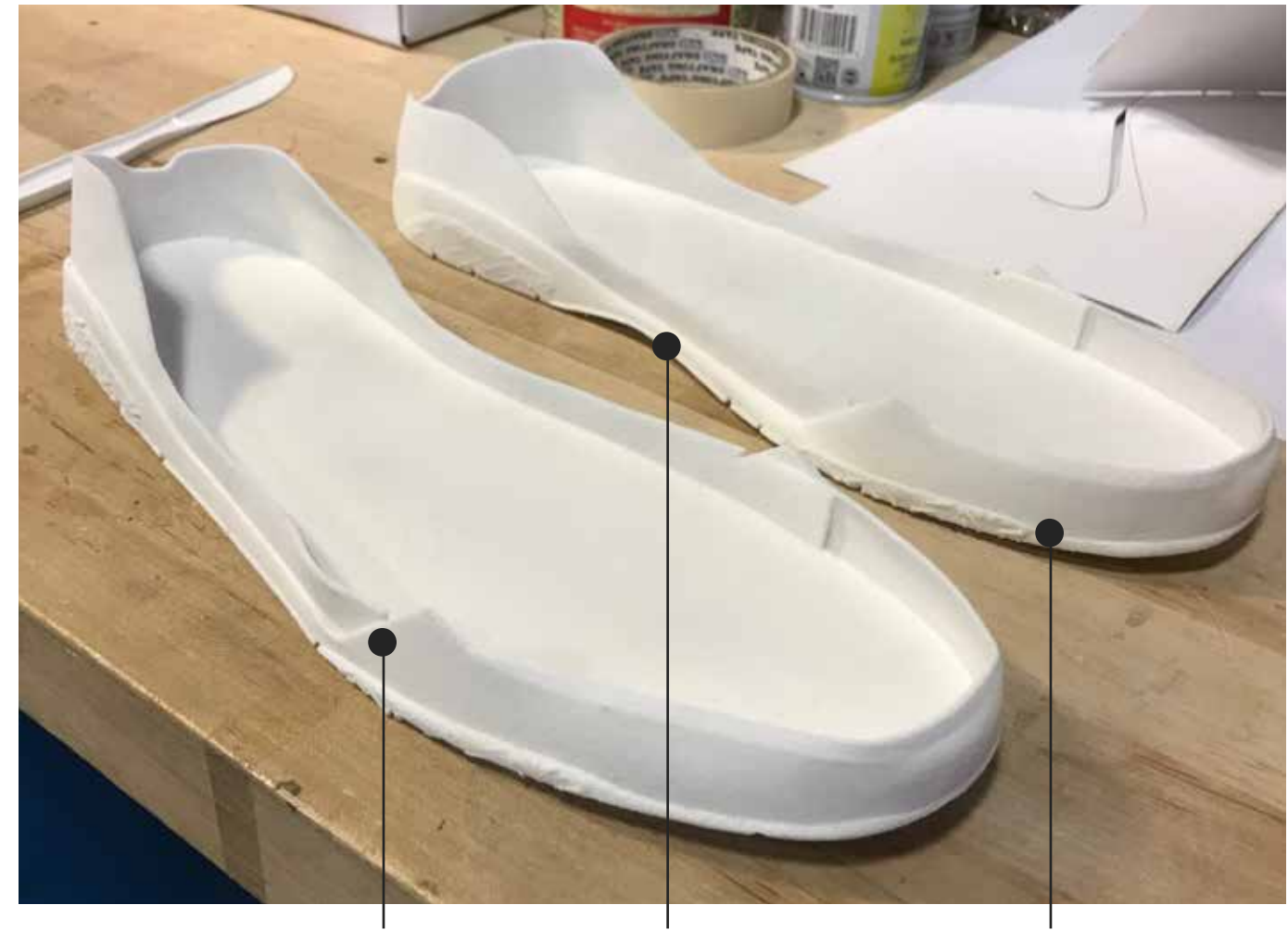
Flex grooves for lateral and medial Medial arch cup for stability Grip along front sidewall for forefoot impact flicking and lateral stability
