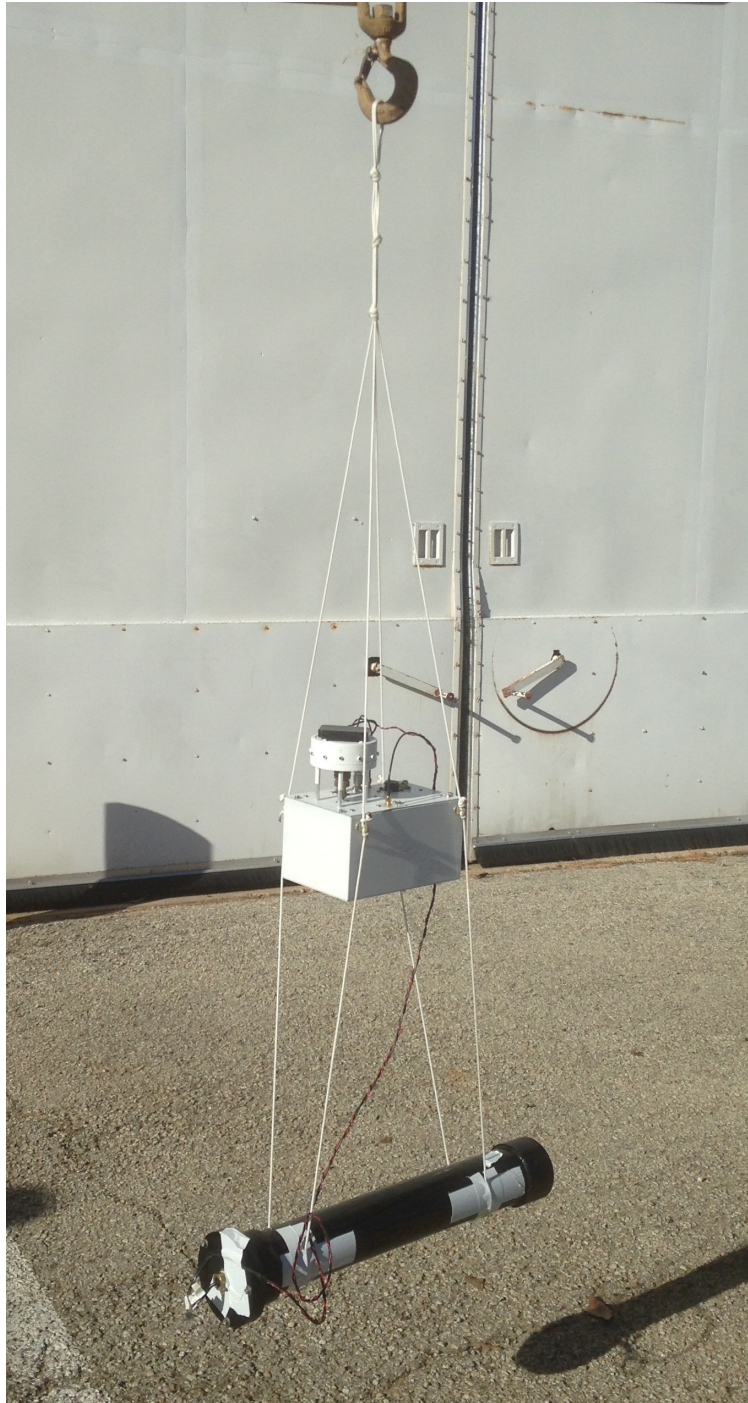
Figure A.14: The hang test at CSBF, where all systems performed nominally, verifying payload-readiness for the Antarctic flight.
