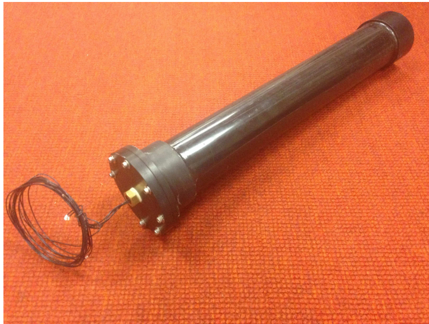
Figure A.11: The HiCal-2 pressure vessel. 9 cm in diameter by 60 cm in length.
