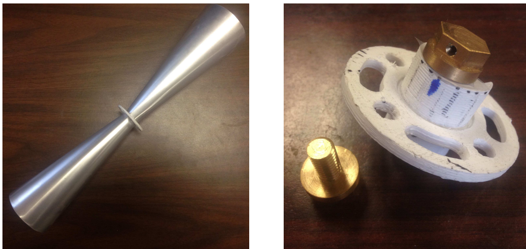
Figure A.9: The HiCal-2 bicone antenna, left, with a detail of the 3d-printed spacer and machined spark gap set bolt, right.
