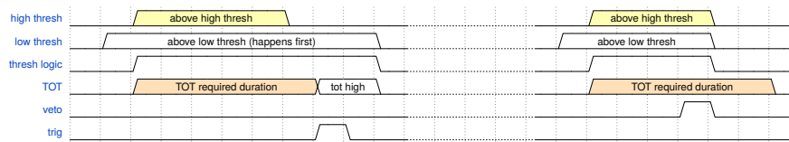
Figure 3.6: example timing diagrams of the trigger system. Left: The trigger envelope rises above low threshold then high threshold. After some amount of time, the time-over-threshold is satisfied, and the trigger goes high. the veto in this case stays low, indicating that there is not a transient present. Right: The trigger envelope rises above the low threshold and also the high threshold, but the veto goes high, which sends the threshold and time-over-threshold logic low, and so the trigger never goes high.
