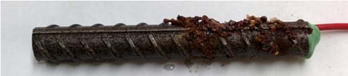
Figure 64 — Rapid macrocell test, anode bar of as-received MMFX(4%)-6 after 15 weeks
