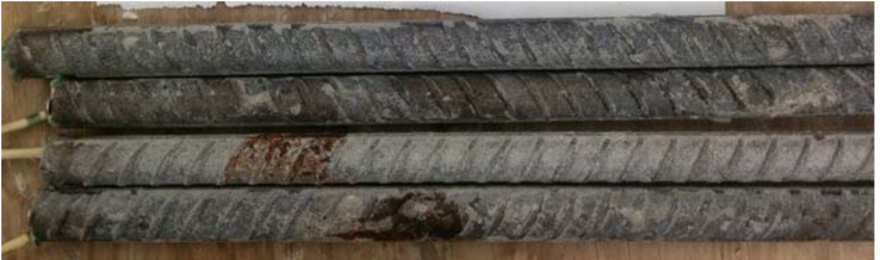
Figure 25 — Southern Exposure MMFX(4%)-6 bottom bars after 96 weeks
