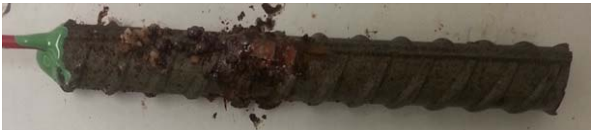
Figure 66 — Rapid macrocell test, anode bar of pickled PMMFX(4%)-4 after 15 weeks
