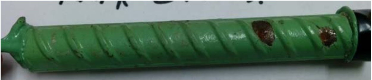
Figure 67 — Rapid macrocell test, anode bar of MMFX-ECR(4%)-5 after disbondment test after 15 weeks
