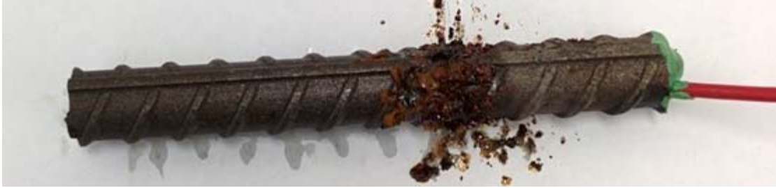
Figure 63 — Rapid macrocell test, anode bar of as-received MMFX(9%)-6 after 15 weeks
