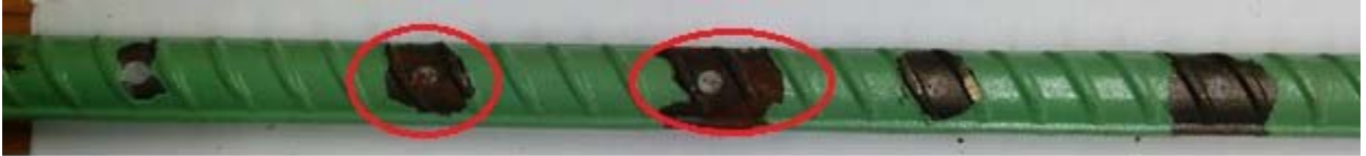
Figure 53 — Cracked beam MMFX-ECR(4%)-5 top bar after disbondment test after 96 weeks
