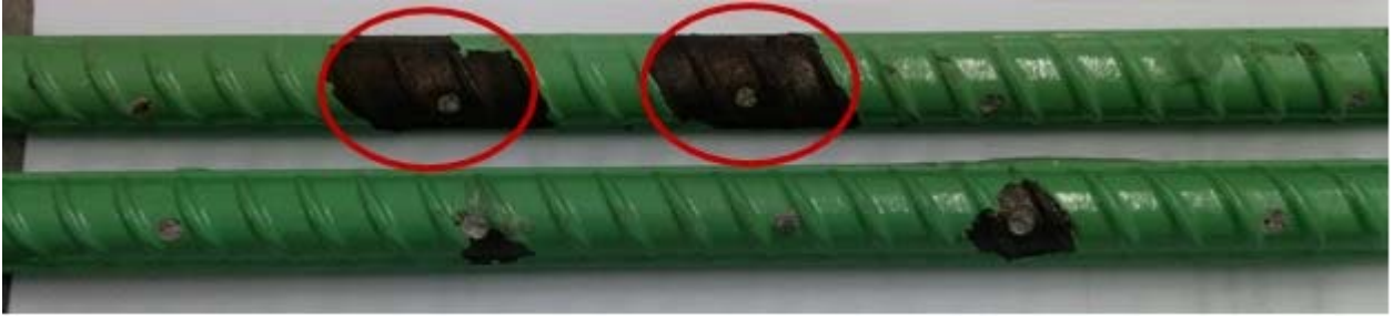
Figure 29 — Southern Exposure MMFX-ECR(4%)-5 top bars after disbondment test after 96 weeks
