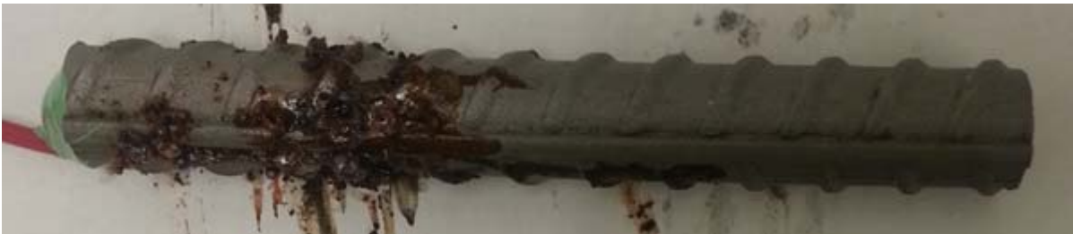
Figure 65 — Rapid macrocell test, anode bar of pickled PMMFX(9%)-3 after 15 weeks
