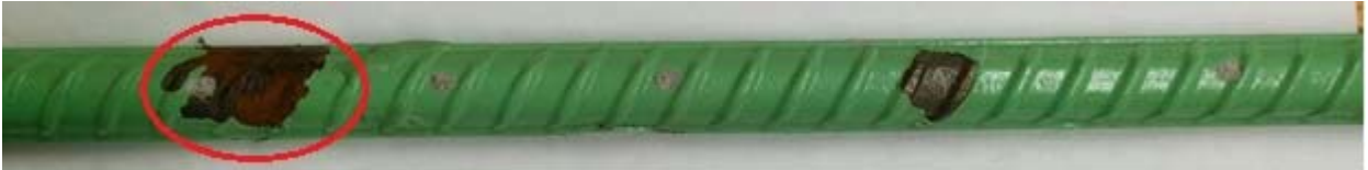
Figure 54 — Cracked beam MMFX-ECR(4%)-5 bottom bar after disbondment test after 96 weeks
