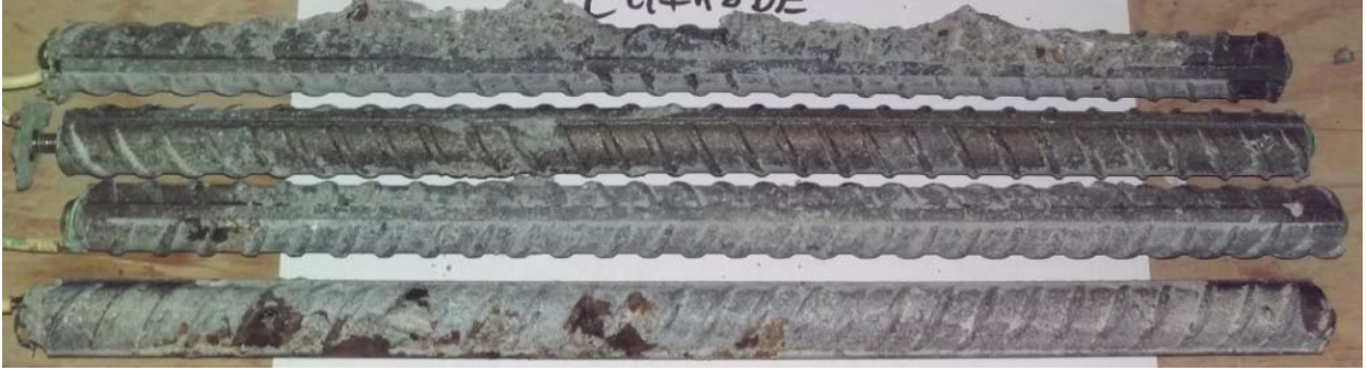
Figure 27 — Southern Exposure MMFX(9%)-5 bottom bars after 96 weeks
