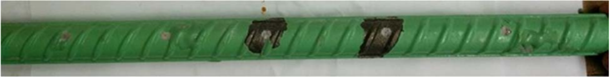
Figure 30 — Southern Exposure MMFX-ECR(4%)-5 bottom bar after disbondment test after 96 weeks
