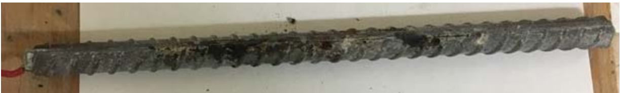
Figure 50 — Cracked beam MMFX(9%)-5 top bar after 96 weeks
