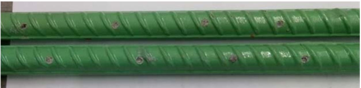
Figure 28 — Southern Exposure MMFX-ECR(4%)-5 top bars before disbondment test after 96 weeks
