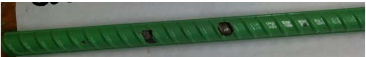
Figure 52 — Cracked beam MMFX-ECR(2%)-2 bottom bar after disbondment test after 96 weeks
