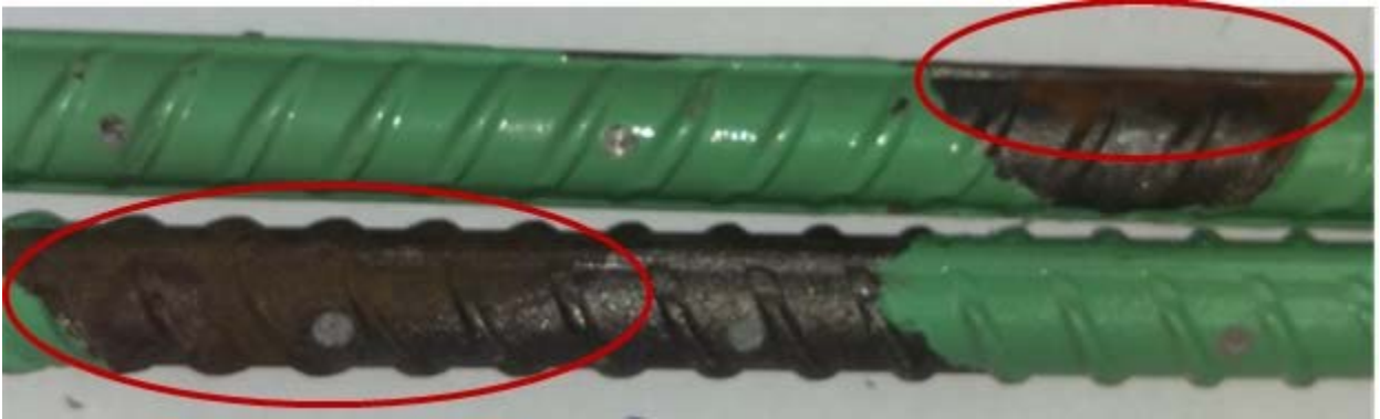
Figure 31 — Southern Exposure MMFX-ECR(2%)-5 top bars after disbondment test after 96 weeks
