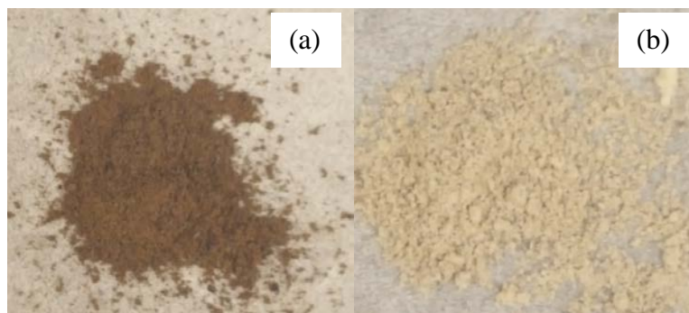
Figure A-20 (a) Catalyst calcined in stable air. (b) Catalyst calcined in N 2 flow
