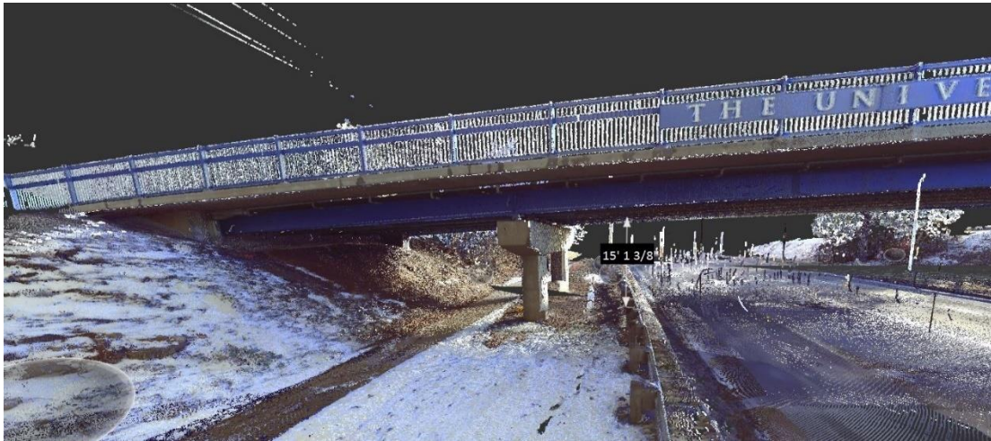
Figure 5.6b: Minimum vertical clearance from scan data
