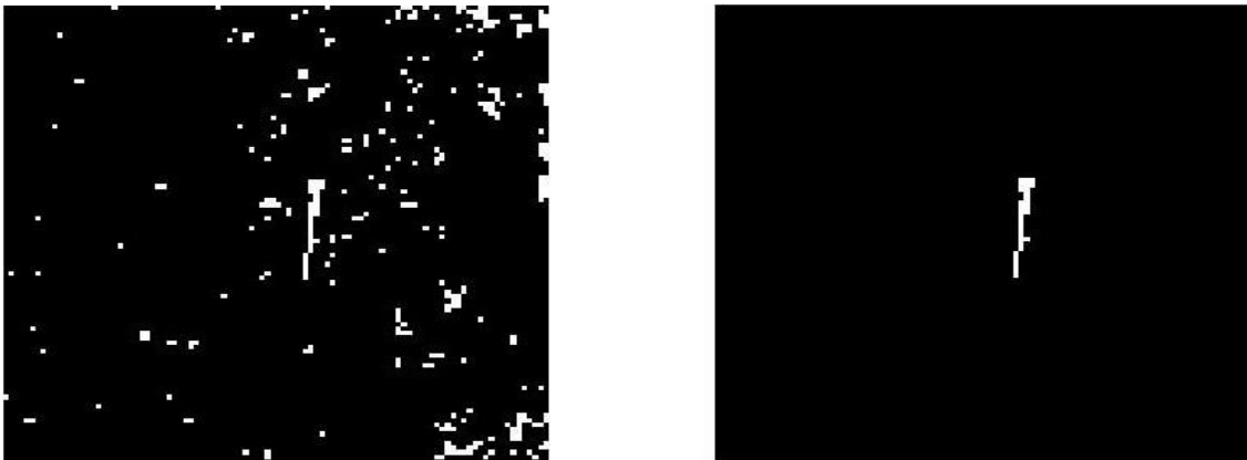
Figure 5.26: ProcessedImage with texture noise(left) and ProcessedImage after noise removal(right)
