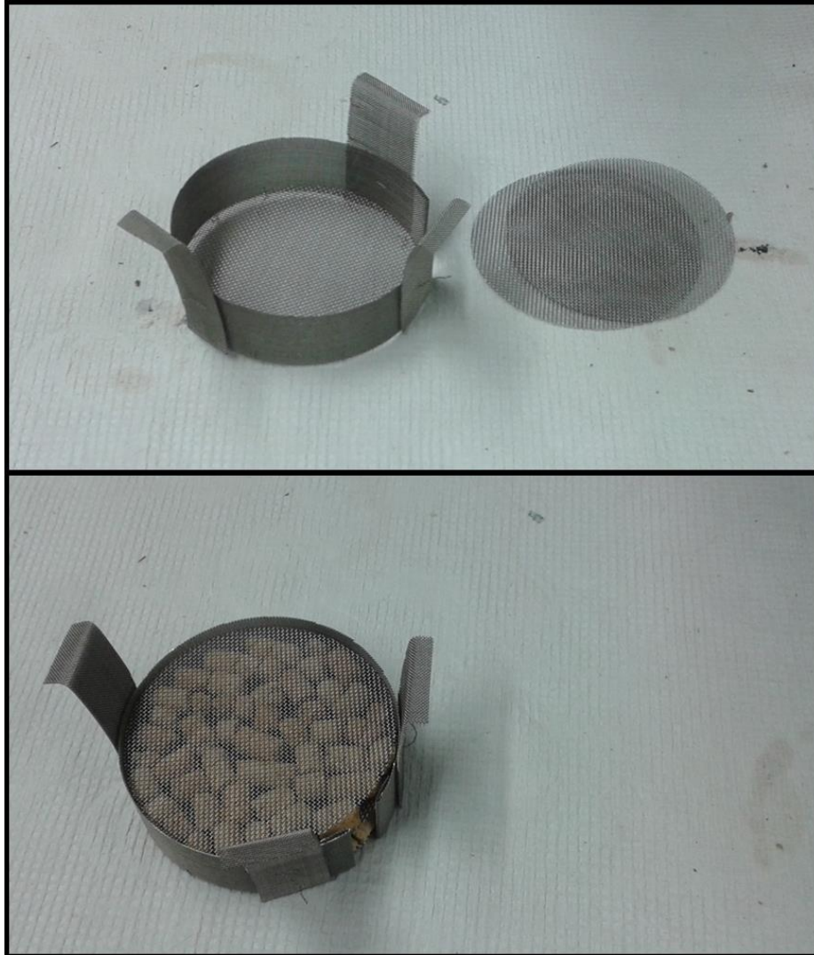
Figure 6 (Top) Angled view of a steel mesh sample basket. The mesh circles to the right of the basket are the mesh "separators," meant to reduce the ash lost to the upwards air flow in the combustor. (Bottom) A fully assembled sample basket. Note that the top separator sits nearly flush with the top of the basket sides.
