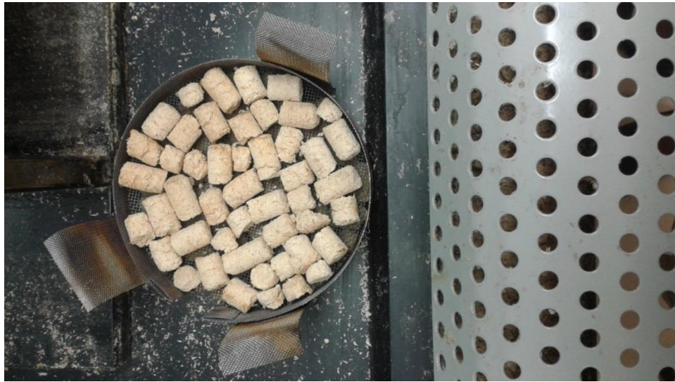
Figure 8 A top down view of a pellet layer within a sample basket.
