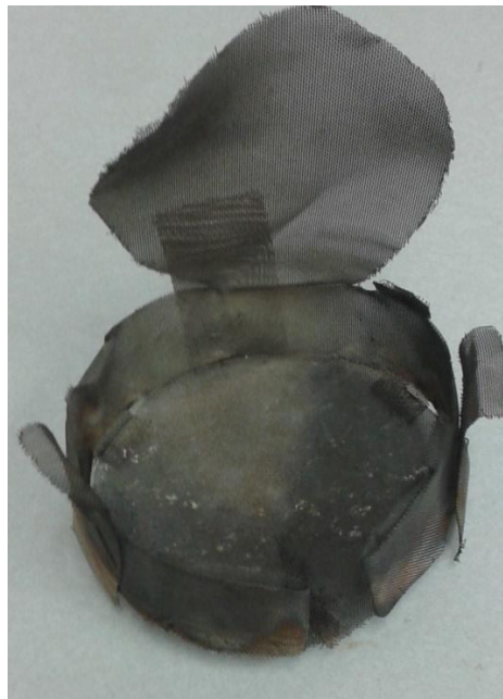
Figure 7 The pre-burn basket. The single piece construction makes precision sizing more difficult, but also increases durability.
