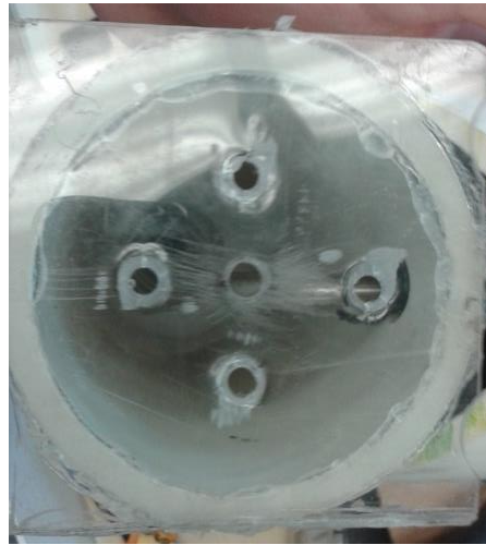
Figure 3 The Plexiglas restrictor plate attached to the end of the flow validation set up.
