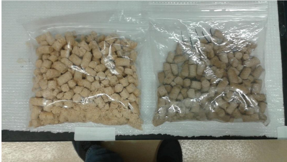
Figure 15 Pure pine pellets (on the left) exhibit higher friability through an increased number of small pieces and dust than the 75%/25% pine/algae pellets (on the right).
