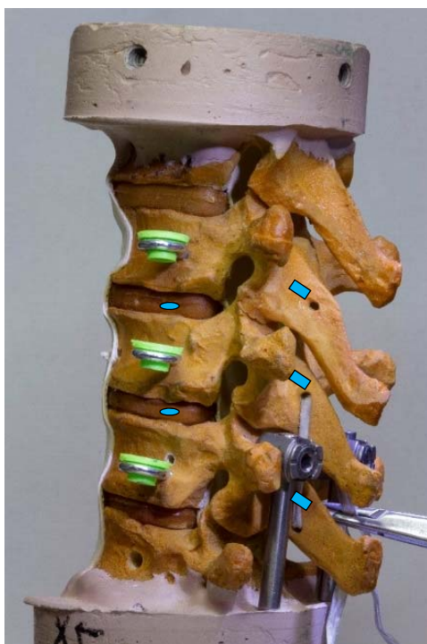
Figure 3.3.1: Model showing an example of a prepared T6-T10 segment. Pressure sensors are indicated by the blue ovals at UIV/UIV+1 and UIV+1/UIV+2 intervertebral discs, and spinous process strain gages are indicated by the blue rectangles at UIV, UIV+1, and UIV+2.
